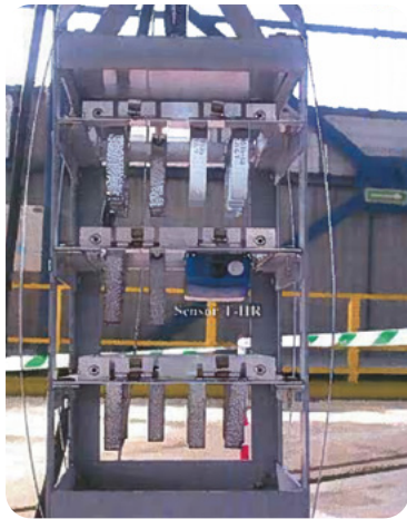
Figure 5-14: Specimens for the study of corrosivity inside the Vandellós I caisson; specimen exposed to corrosion for five years increased 2,500 times
