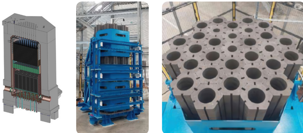
Figure 5-16: 3D model of the Vandellós I reactor caisson and models of the graphite stack in the industrial demonstrator
