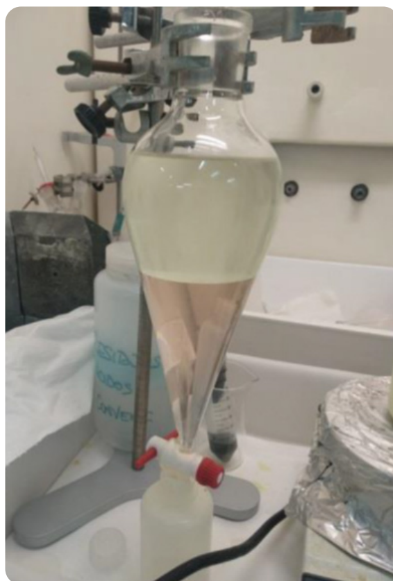
Figure 5-17: Separation of \text{UO}_2(\text{NO}_3)_2 \cdot 6\text{H}_2\text{O} by decantation. Colour change of the phases as a function of the amount of uranium remaining in them
