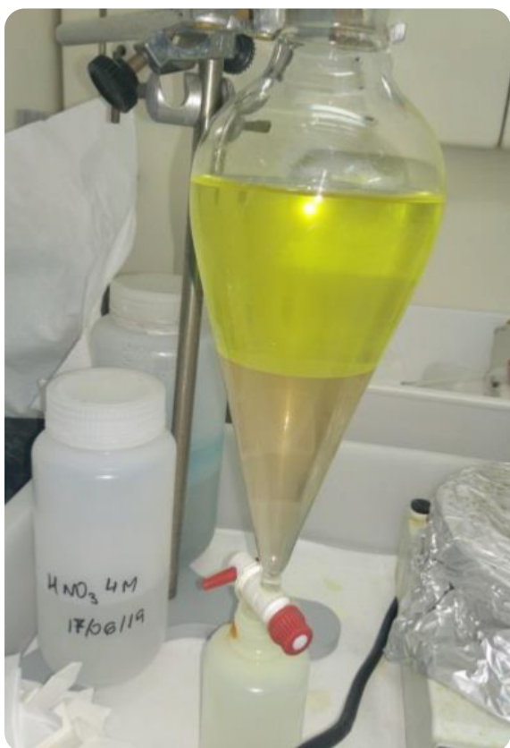
Figure 5-17: Separation of \text{UO}_2(\text{NO}_3)_2 \cdot 6\text{H}_2\text{O} by decantation. Colour change of the phases as a function of the amount of uranium remaining in them
